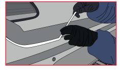
For best results remove before clear coat bake. Stretch the tape when de-masking to ensure clean removal.
