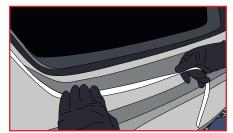
Choose required contour to blend to and apply directly to vehicle ensuring tape is not stretched.
